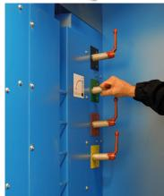
The group of nozzles is controlled using buttons (left picture) or "ball valves" (right picture). The control elements and group of nozzles are identified by colours. The control elements have the same colour as the respective group of nozzles. Thereby, there is clear allocation, because either the complete working clothing can be purged, or only a part of it.
